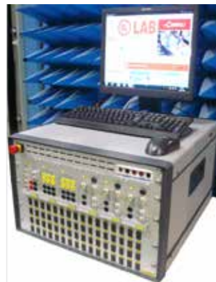
Example of automatic data acquisition system rack
